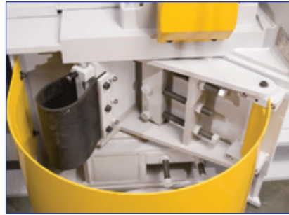
Shear pin protected anvil door
