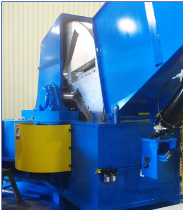
Cylinder-operated quadrant opening
