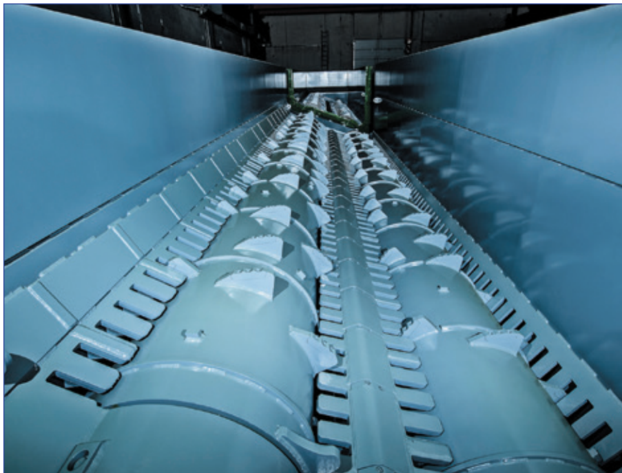
Tight tolerances between the debarking blocks and comb teeth ensure maximum retention of useable fiber
